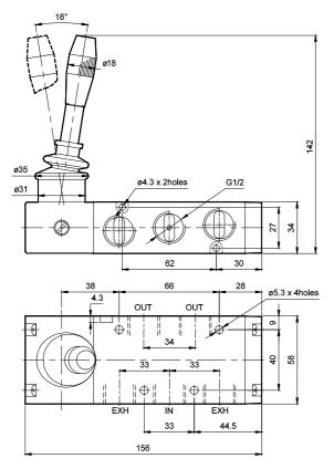
5 / 3 Hand lever operated valve with detent
